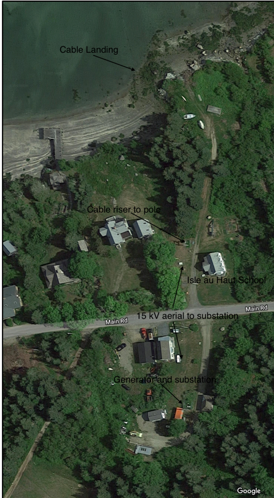
Fig. 5. Cable landing and POCO substation. 44.07654,-68.631170 Isle au Haut Solar + Storage Islanding Minigrid Request for Proposals
